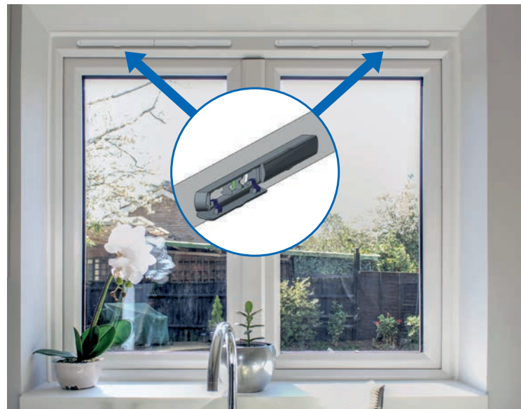
Trickle Vents installed through the outer frame Also showing the functionality of the internal link vent closure plates
